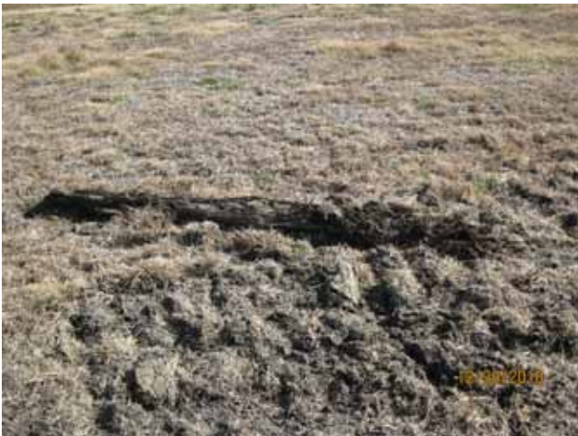
4. Issue: Unsuitable material in processing area on protected side of levee. GPS Coord: 2953.227 N 09008.606 W to 2953.249 N 09008.626 W
